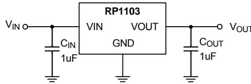
**Note:** To prevent oscillation, a 1µF minimum X7R or X5R dielectric is strongly recommended if ceramics are used as input/output capacitors. When using the Y5V dielectric, the minimum value of the input/output capacitance that can be used for stable over full operating temperature range is 3.3µF. (see Application Information Section for further details)
